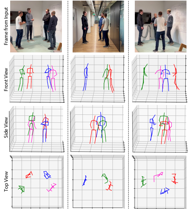
Figure 5. Qualitative results on an in-the-wild setting predicted by MuPPet. We show one frame from the video input and corresponding three views of the predicted 3D pose from multiple persons in the scene. Our MuPPet demonstrates effective performance in absolute 3D joint prediction, even on highly occluded persons.
