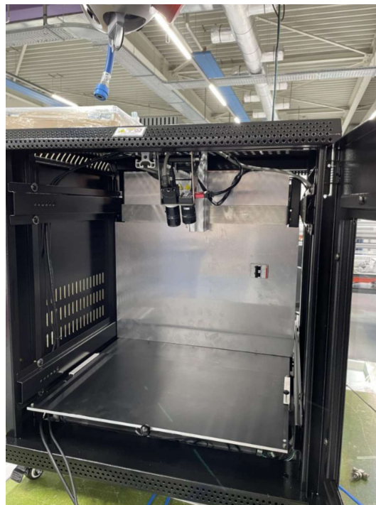
Figure 5. 3D Quality Control Setup developed by Sioux Technologies [24]. This setup leverages event-camera technology to provide fast, high-fidelity 3D scanning suitable for in-line real-time quality assurance for specialized products. It aims to deliver optimized process control in applications including 3D metal printing, integrated electronics in molded parts, and dental prosthetics.
