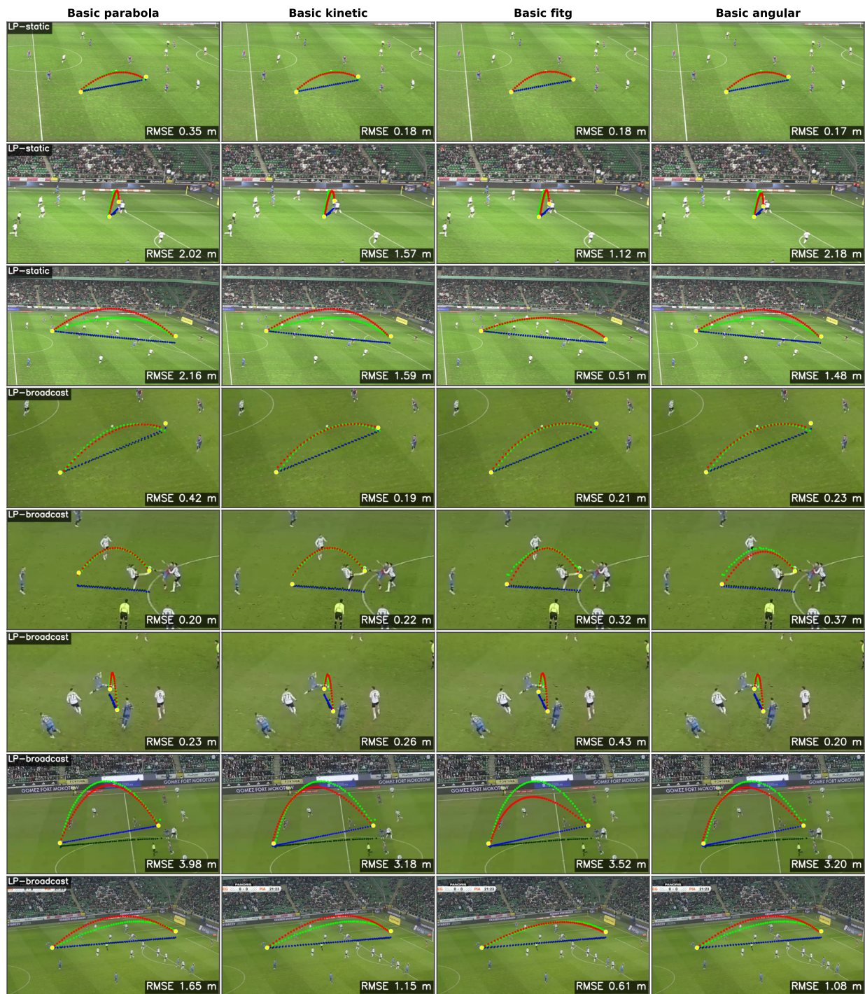
Figure 3. Qualitative model comparison on the Legia-Piast dataset (static and broadcast cameras). Each column corresponds to one physics model (Table 1). Visualization: red dots show the predicted 3D trajectory projected onto the video frame; green dots show the oracle 3D ground truth; blue and dark-green dots show the corresponding pitch-plane (ground) projections of the prediction and ground truth, respectively; yellow markers indicate segment endpoints (pivot points). Per-panel 3D RMSE in meters is overlaid in the bottom-right corner; the dataset and camera type are indicated in the top-left corner of the first column.
