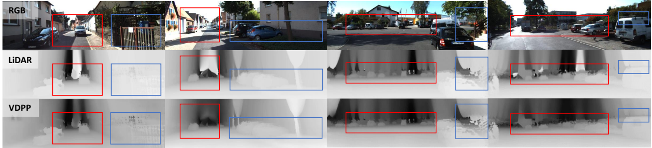
Figure 3. Qualitative validation of VDPP on real-world LiDAR data from the KITTI dataset [4]. We compare the “Raw Inpainted” depth (from LiDAR depth completion) against our refined “VDPP” output across four driving sequences. The red boxes highlight VDPP’s ability to suppress artifacts inherent to the inpainting process, such as horizontal streaking. The blue boxes demonstrate how VDPP enhances depth expression , clarifying object boundaries and improving geometric detail where the raw input was poorly defined. This validation confirms VDPP is not limited to refining single-image models but also serves as a powerful plug-and-play post-processor, significantly improving depth quality from real-world 3D sensor pipelines.
