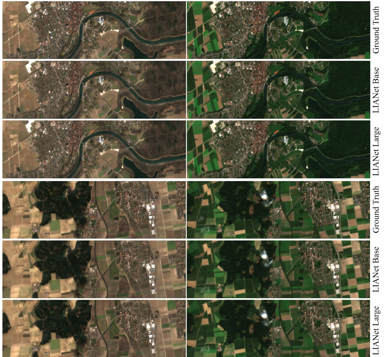
Figure 6. Two examples of reconstruction quality of LIANet-Base and LIANet-Large on \mathcal{A}_0 area. It can be seen that LIANet-Large has an improved performance in reconstructing the high-frequency details, including buildings within the city. It can also be seen that cloudy areas are reconstructed as they are present in the Sentinel-2 image.
