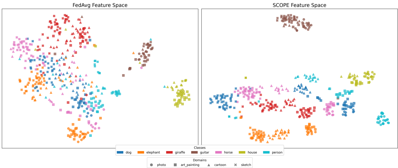
Figure 1. t-SNE visualization of feature spaces from the final shared trunk layer, evaluated on the PACS dataset. Colors correspond to semantic classes and marker shapes correspond to source domains. (Left) The FedAvg baseline learns an entangled representation where classes and domains are heavily mixed. (Right) The SCOPE framework learns a superior representation with distinct, compact class clusters that are demonstrably invariant to the source domain.
