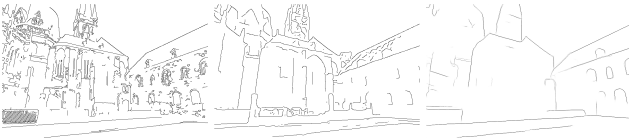
Figure 4. Examples of the used edge extraction methods. From left to right: Canny edge detector used directly on the image, Canny edge detector applied on a Metric3D depth map, and an edge map extracted with DiffusionEdge.
