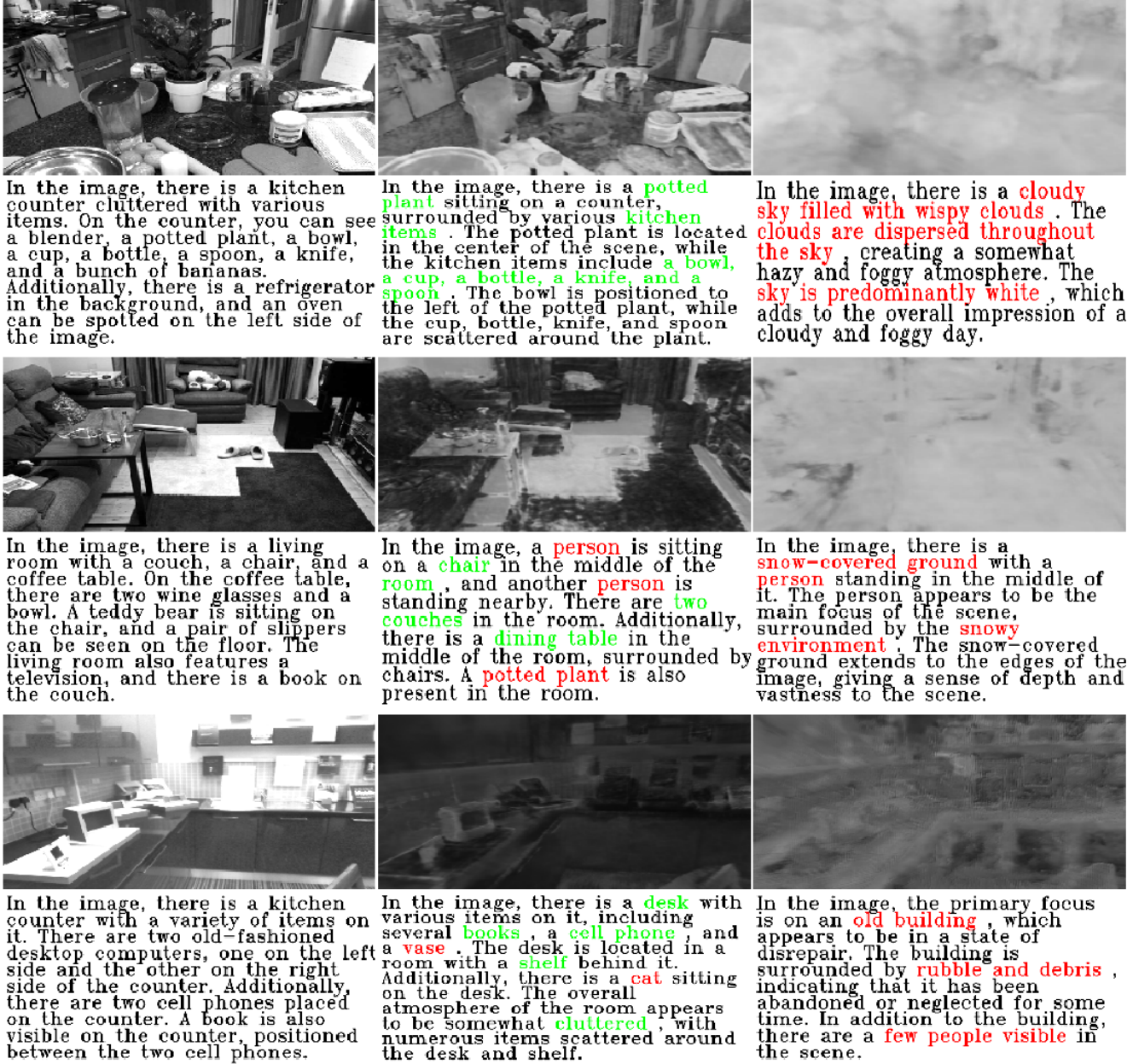
Figure 3. From left to right: Ground truth image, image reconstructed from ZipNeRF-wo-RGB, image reconstructed from ppNeSF with the inversion attack. Below each image we show the associated LLaVa’s descriptions highlighting in green objects correctly identified by the VLM and in red hallucinated objects.
