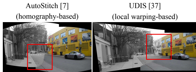
Figure 2. Conventional panoramic image stitching methods [8, 44] fail to account for strong parallax or variations in lighting or style.
