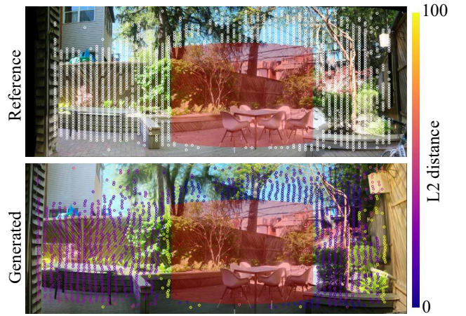
Figure S6. Example of LoFTR feature matching between reference and generated panoramas. White circles mark selected keypoints in the reference, with corresponding points in the generated panorama color-coded by L2 pixel distance from their reference positions.
