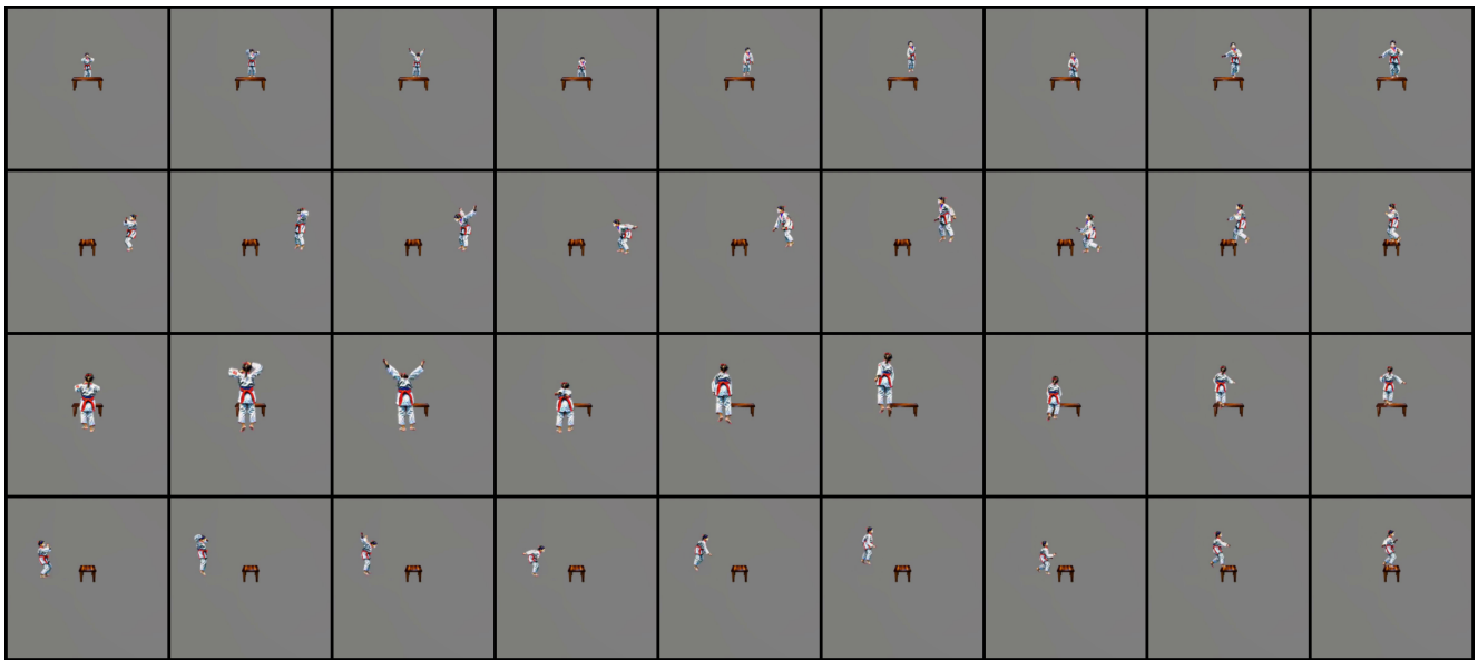
Figure 6. Generated motion for the prompt: "the human prepares to jump for 1 second then jumps onto the table and stops on the surface of the table for 1 second". Top: 4Df. Bottom: MSDI. The four rows illustrate the motion from different camera viewpoints
