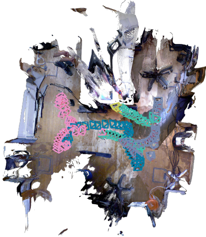
Figure 4. Preservation of geometric cues in the DEMs, alongside semantics help in accurate trajectory estimation in planar scenes like the TUM RGB-D floor scene as shown in the figure.
