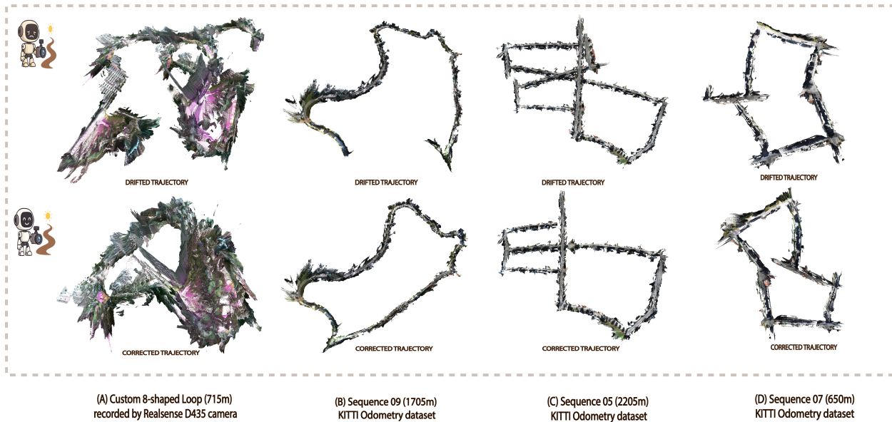
Figure 1. VGGT-SLAM++ provides an end-to-end SLAM architecture that stabilizes transformer-based odometry by using a low-fidelity geometric representation to support a high-cadence optimization back-end. The trajectories in the upper row are the odometry based trajectories while the lower row corresponds to the corrected trajectories when stabilised by our back-end.
