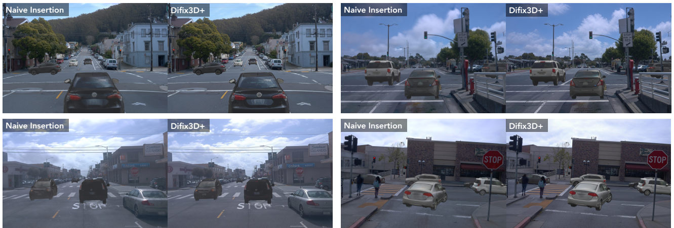
Figure 9. Samples of Difix3D+ [43] applied on the R3D3 dataset. The model sharpens the image, saturates the colors, adds contrast and improves the look of the vehicle but it does not attempt to add any shadows or realistic light effects.
