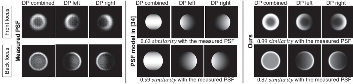
Figure 5. Front and back focus DP PSFs. The similarity between two PSFs is measured by the 2D cross correlation. **Left:** Measured DP PSFs from the Canon 5D Mark IV DSLR. **Middle:** DP PSFs as modeled by [34]. **Right:** Our newly proposed model for DP PSFs based on a modified 2D Butterworth filter. Our modeling achieves higher correlation with the real-world measured PSFs.
