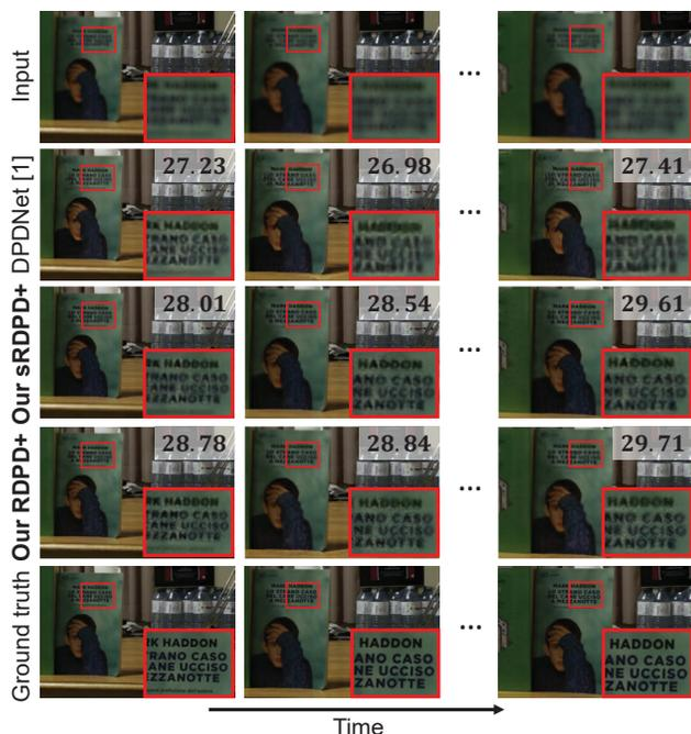
Figure 8. Results on a Canon 5D DSLR image sequence. PSNR is shown for each deblurred image. sRDPD+ has a 0.4dB lower PSNR on average when it is trained with a single frame compared to our multi-frame method – that is, RDPD+.
