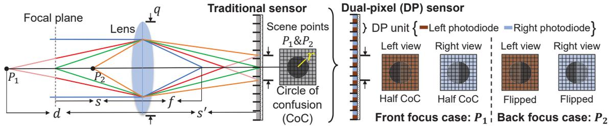
Figure 2. Thin lens model illustration and dual-pixel image formation. The circle of confusion (CoC) size is calculated for a given scene point using its distance from the lens, camera focal length, and aperture size. On the two dual-pixel views, the half-CoC PSF flips if the scene point is in front or back of the focal plane.
