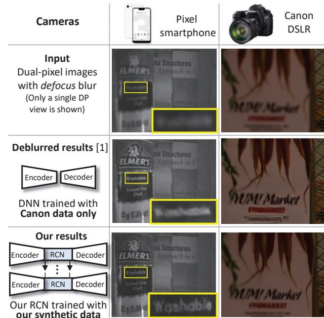
Figure 1. Deblurring results on images from a Pixel 4 smartphone and a Canon 5D Mark IV. **Third row:** results of the DNN proposed in [1] trained with DP data from the Canon camera. **Last row:** results from our proposed network trained on *synthetically generated data only*.
