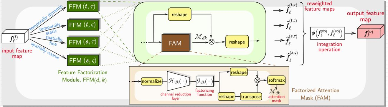
Figure 2: **Overview of STRF module.** Our proposed module contains four factorization units being applied on input feature volume at  $\ell$ th layer to extract static/coarse and dynamic/fine information and generate richer feature representation. Each unit is composed of a Feature Factorization Module aided by the proposed Factorized Attention Mask block.
