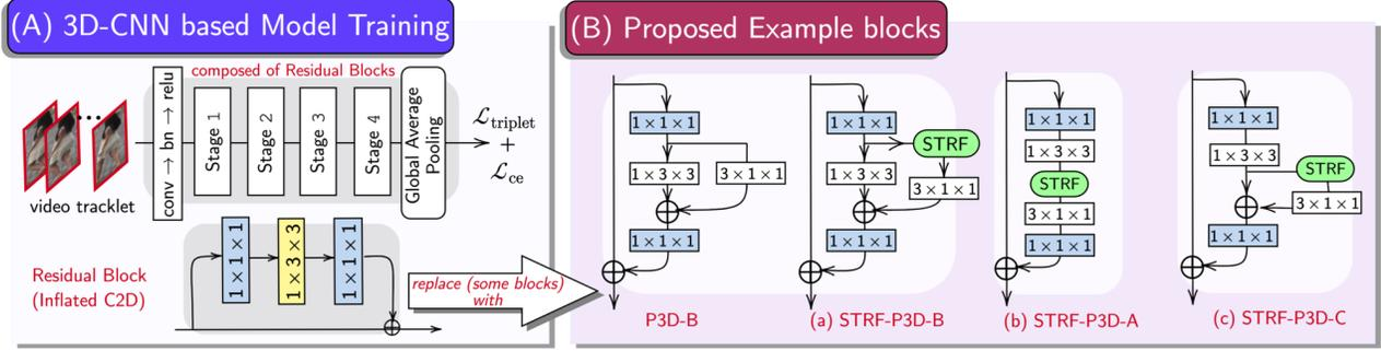
Figure 3: **Illustration of our 3D-CNN model training and examples of proposed blocks.** In our framework, we employ a 3D-CNN based model to learn discriminative features for input video tracklets (see Figure (A)). This model is built with inflated 2D-residual blocks with Stage 2 and Stage 3 replaced by our proposed STRF aided residual blocks (see Figure (B)).
