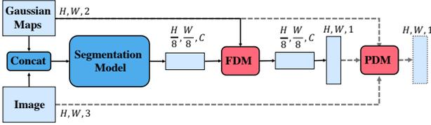
Figure 2. An overview of our Conditional Diffusion Network. FDM denotes Feature Diffusion Module. PDM denotes Pixel Diffusion Module. The dotted lines mean PDM only exists during inference.
