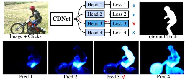
Figure 5. Demonstration of Diversity Training. We predict  $N$  more potential results and chose the one most similar to the ground truth to propagation the gradients. The original head is not shown for simplicity.
