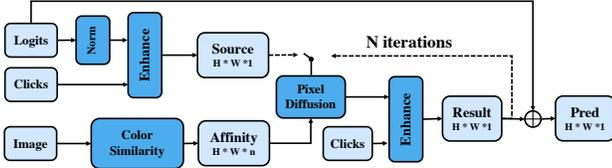
Figure 4. Pipeline of Pixel Diffusion Module (PDM). PDM takes the original image, Gaussian maps of clicks, and the predicted logits as input. It propagates information from clicks to neighbors iteratively to get the refined prediction map.
