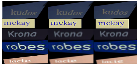
Figure 7: Results of BPN simulation. From top to bottom, transforms applied are identity, sharpening, motion blur, and two different levels of isotropic Gaussian blur. Left, middle and right columns indicate input, blur model output, and BPN output.
