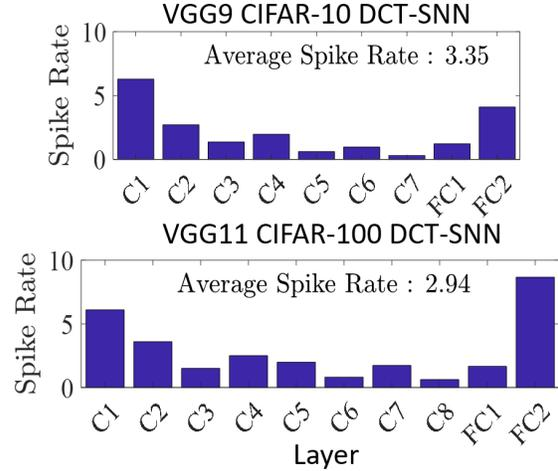
Figure 7: DCT-SNN layerwise spike rate. C and FC denote Conv and Fully Connected layers, respectively.
