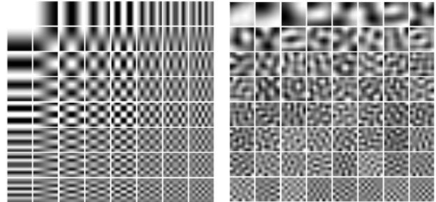
Figure 3:  $8 \times 8$  2-D DCT bases (left) and PCA bases for CIFAR-10 (right). The DCT bases are ranked in a zig-zag fashion starting from top left to the bottom right and the PCA bases are ranked from left to right and top to bottom.
