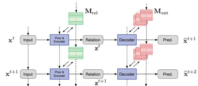
Figure 1. Memory-augmented dynamic neural relational inference. The prior/encoder term is used to dynamically estimate the relation type distribution  $\mathbf{z}^t$  for each step, which is used to predict the future via the decoder. We use dual memory pools and the corresponding memory modules to maintain the long-term temporally global information of the relations and entities.
