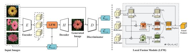
Figure 1: Our LoFGAN framework contains an encoder E, a local fusion module, a decoder H, and a discriminator D. The random coefficient vector  $\alpha$  is the input of both LFM module and local reconstruction loss. The local fusion module randomly chooses one of the encoded features as base and the rest features as references, and fuses them by local selection, local matching and local replacement.
