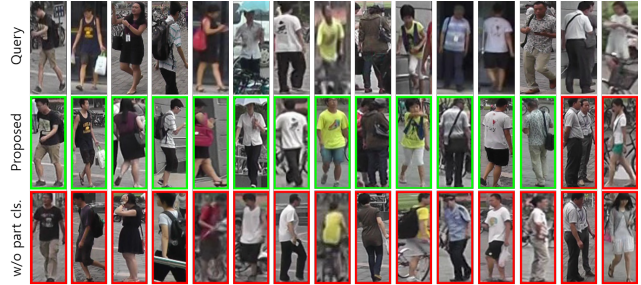
Figure 6: Qualitative comparison results with and without part classification. The results of true and false matching are depicted in green and red, respectively.
