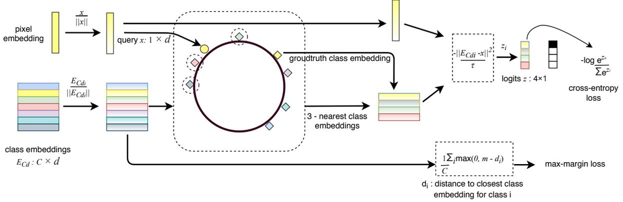
Figure 3. **Loss Computation:** A pixel embedding  $x$  and class embedding  $E_{Cd}$  are normalized to project on a hyperspherical manifold. For normalized  $x$ ,  $k=3$  nearest class embeddings are searched (shown by dotted circle). L2 distance between normalized  $x$  and class embeddings is used to compute logits for  $k$  negative nearest classes and a positive class. Further, classification and regularization loss is computed.
