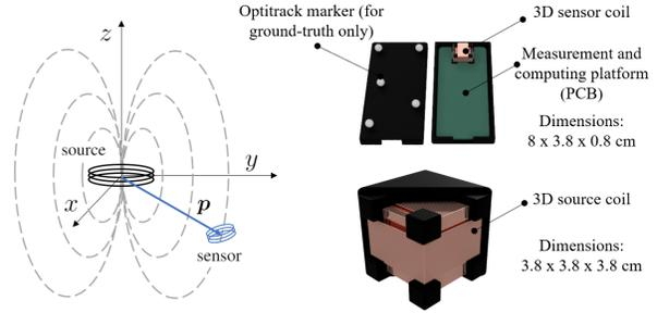
Figure 2: **EM sensing.** (left) A 1D coil is generating a magnetic B-field. Another coil can solve for its position  $\mathbf{p}$  w.r.t. the source by comparing measured and theoretical voltage. (right) Schematics of our source and sensors.
