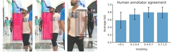
Figure 3: We visualize bounding boxes labeled by multiple (4) in-house annotators (left). During small occlusions, annotators strongly agree. During large occlusions (less than 10% visible, last frame), annotators still agree to a fair extent (average IoU overlap of 60%, right), but require temporal video context. We use these to justify our Top- $k$  evaluation and motivate our probabilistic tracking approach.
