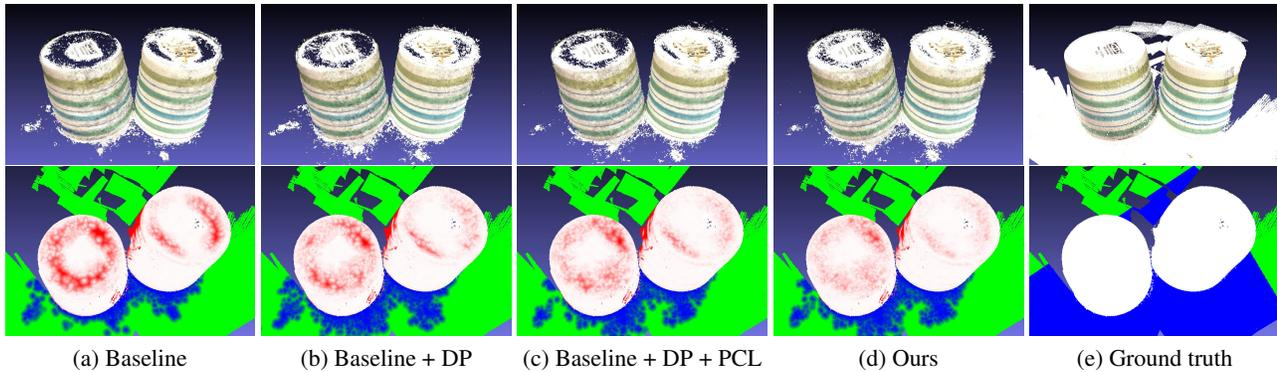
Figure 8: Qualitative ablation study on *scan48* of the DTU dataset. The 1st row shows the 3D reconstruction results of (a) baseline, (b) baseline with double prediction (DP) layers, (c) the aforementioned model with the 3D Point Consistency Loss (PCL), and (d) our integrated method with Coarse-to-fine Reliable Depth Propagation. The 2nd row shows the error maps of the reconstruction results and red color represents the severity of the errors.
