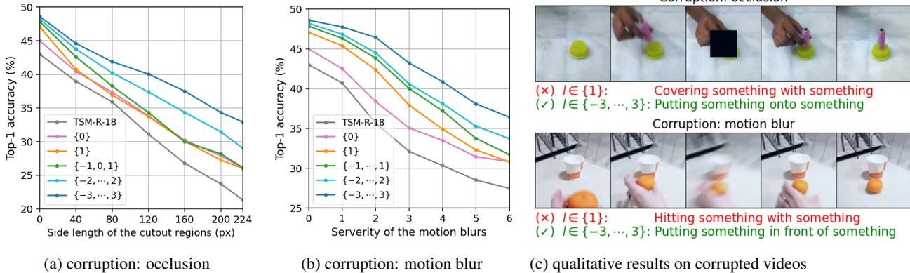
Figure 5: **Robustness experiments.** (a) and (b) show top-1 accuracy of SELFYNet variants (Table 4a) when different degrees of occlusion and motion blur, respectively, are added to input. (c) shows qualitative examples where SELFYNet ( $\{-3, \dots, 3\}$ ) succeeds while SELFYNet ( $\{1\}$ ) fails.
