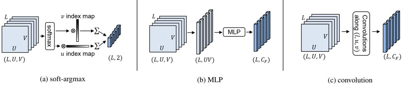
Figure 3: **Feature extraction from STSS.** For a spatio-temporal position  $(t, x, y)$ , each method transforms  $(L, U, V)$  volume of STSS tensor  $\mathbf{S}$  into  $(L, C_F)$ . See text for details.
