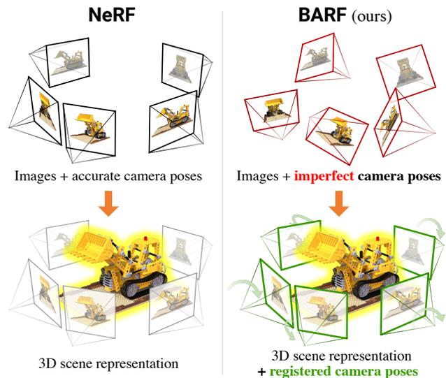
Figure 1: Training NeRF requires accurate camera poses for all images. We present **BARF** for learning 3D scene representations from *imperfect* (or even *unknown*) camera poses by jointly optimizing for registration and reconstruction.
