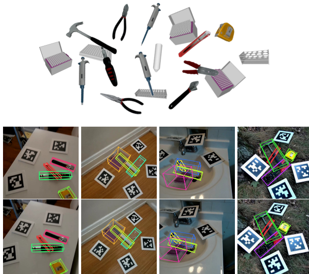
Figure 1: StereOBJ-1M dataset. Upper: CAD models of the objects in the dataset. Lower: four data stereo image pair samples with bounding box annotations.
