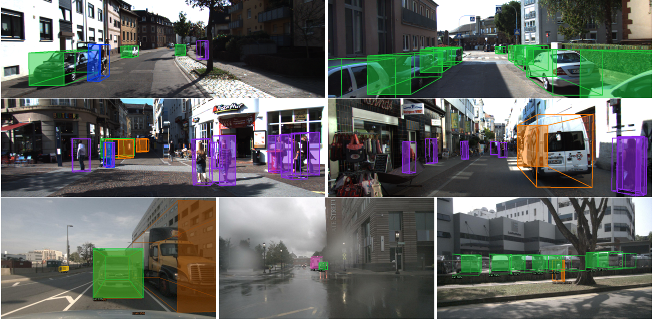
Figure 3: Qualitative visualization of DD3D detections. The first two rows are from the KITTI-3D dataset and the last row is from nuScenes. None of the images were seen during training.
