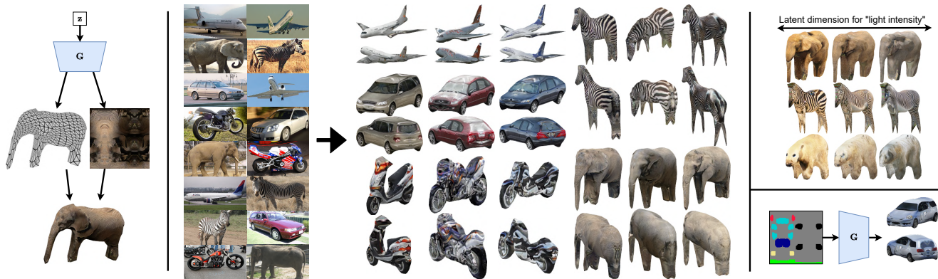
Figure 1. Left: we focus on GANs, where our generator outputs a triangle mesh and a UV-mapped texture. Middle: our method learns to synthesize textured 3D meshes given a real-world collection of 2D images. Top-right: we showcase a setting where we train a single model to generate all classes. This model successfully disentangles some factors of the 3D environment (e.g. lighting/shadows) without explicit supervision. Bottom-right: we also demonstrate a conditional model that generates meshes from 3D semantic layouts.
