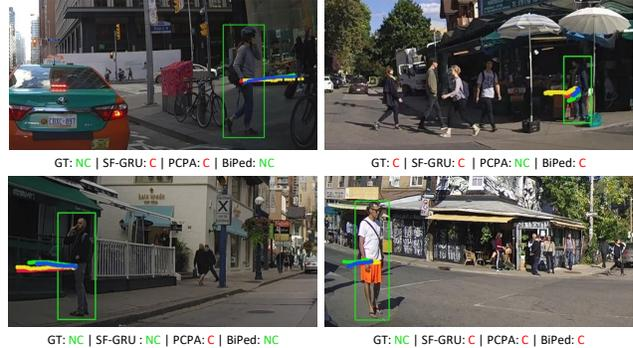
Figure 4. Qualitative results of the proposed algorithm on PIE. Trajectories show one second in future and correspond to **ground truth**, **BiPed (ours)**, **PIE<sub>full</sub>**, and **B-LSTM**. For actions, we report the results on **BiPed (ours)**, **SF-GRU** and **PCPA**. The results correspond to pedestrian crossing (**C**) and not-crossing (**NC**) actions. Here, ground truth is denoted as **GT**.
