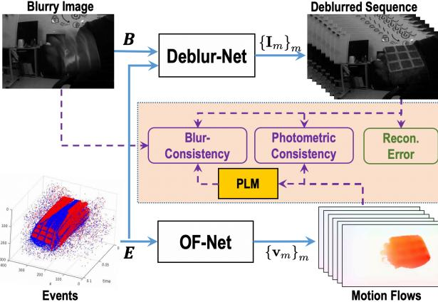
Figure 2. Overview of the proposed learning framework for Real-world Event based motion Deblurring Network (RED-Net), where the blur-consistency and photometric-consistency provide self-supervised losses for real-world datasets and the reconstruction error provides the supervised loss for synthetic datasets.
