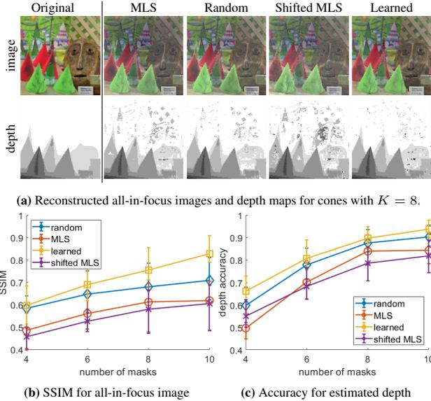
**Figure 3:** Comparison of different types and number of masks. (a) Reconstructed all-in-focus images and depth maps for cones with  $K = 8$  measurements. (b,c) Average SSIM of recovered all-in-focus images and accuracy of estimated depth for five test scenes. Quality of reconstruction improves as the number of masks increases, and learned mask patterns outperform other mask patterns.
