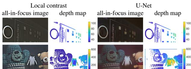
**Figure 8:** The all-in-focus images and depth maps generated by the local contrast-based method and the trained U-Net. Local contrast method uses 47.85 seconds and U-Net uses 0.0043 seconds on average.
