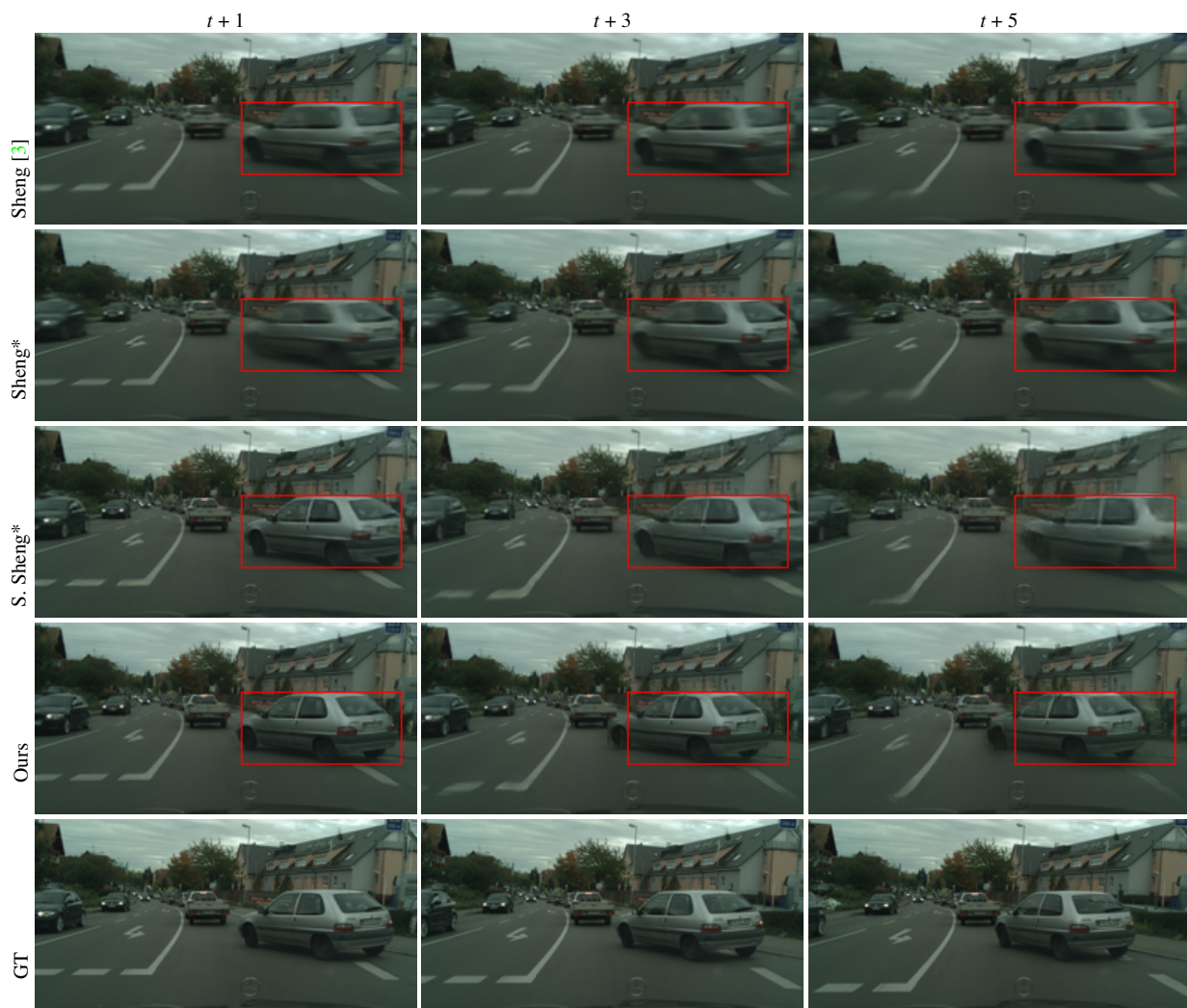
Figure 3: Results of predicting the frames t+1 , t+3 , and t+5 on the Cityscapes dataset [1] with ground truth reference. On first three columns, we move the pedestrian near the semaphore to left. On the last three columns we move car crossing the street. The position of the moved object at t=0 is highlighted in red. Zoom for details.
