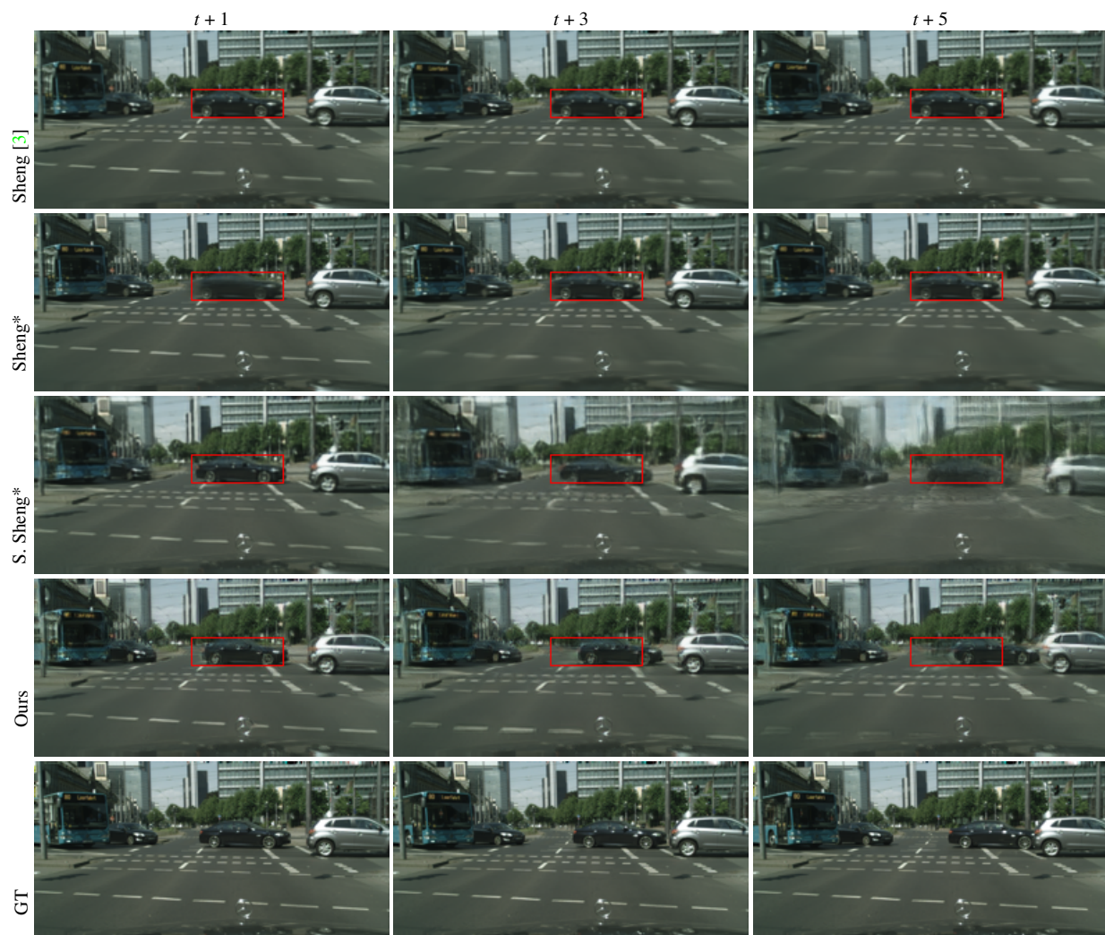
Figure 1: Results of predicting the frames t+1 , t+3 , and t+5 on the Cityscapes dataset [1] with ground truth reference. On first three columns, we move the pedestrian near the semaphore to left. On the last three columns we move car crossing the street. The position of the moved object at t=0 is highlighted in red. Zoom for details.
