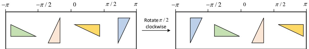
Figure 2. Illustration of random global rotation in range view.
