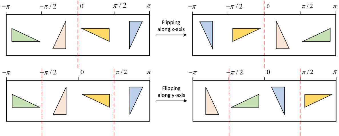
Figure 1. Illustration of random global flipping in range view. Rectangles with black solid line stand for range images. Triangles in the same color indicate an object before and after the augmentation. Red dash lines indicate the flipping axes.
