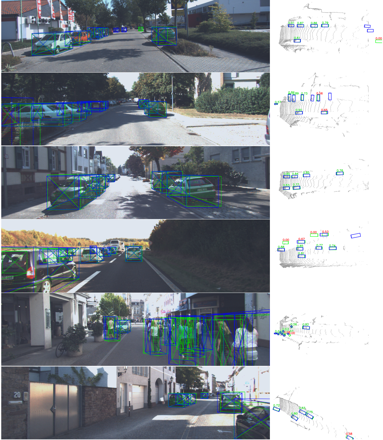
Figure 1. Visualization results of the KITTI validation set. The green boxes are ground-truth 3D / BEV bounding boxes. The blue boxes are our predictions. The numbers around the ground-truth BEV boxes are the IoU values of their best predictions. The IoU values will be zero if the corresponding 3D boxes are not detected.
