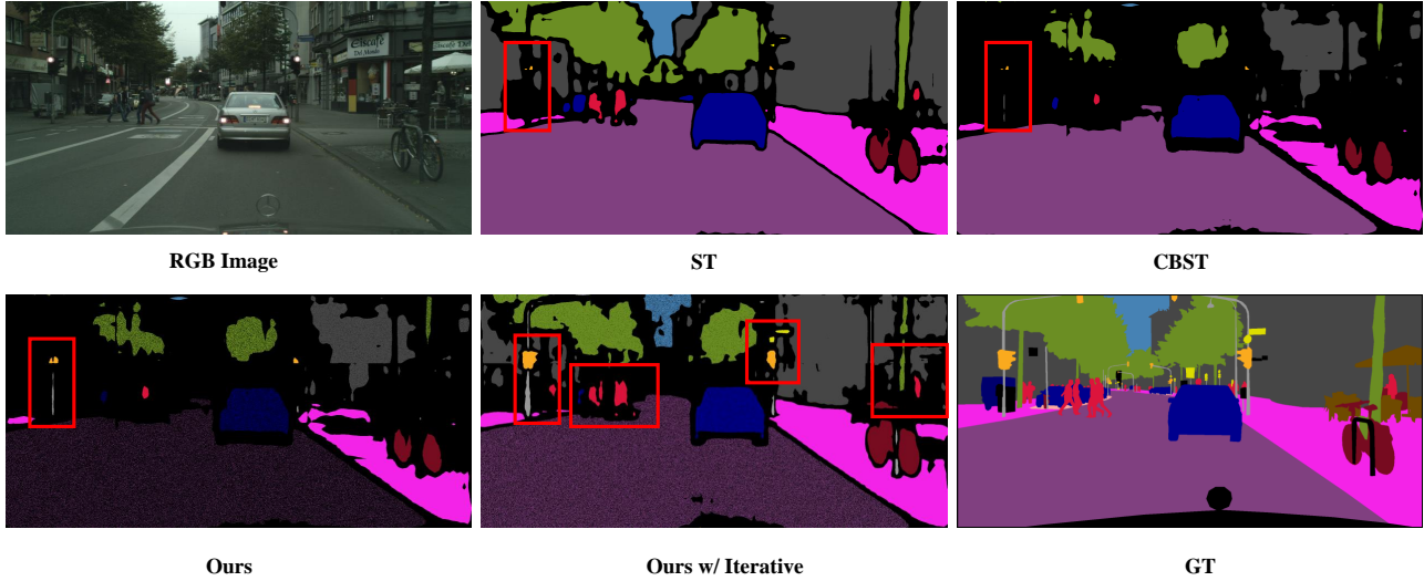
Figure S1. Visualization of pseudo labels generated by different methods. We provide the pseudo labels of ST, CBST and ours at round k=1 (i.e. Ours) as well as ours at round k=2 (i.e. Ours w/ Iterative), together with the RGB image and the corresponding ground-truth. Black areas indicate the ignored region.
