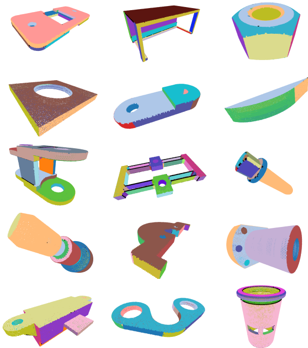
Figure 1. Primitive instance segmentation visualization using our method on ABC dataset.
