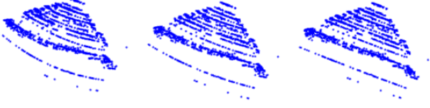
Figure A.1: Resulting 3D reconstruction when no update (left), 1 update (middle), and 2 updates (right) of the linearization with pOSE are performed, for \eta = 0.5 and without reducing \eta in each update. By performing two updates, the reprojection error decreased from 3.57 to 1.48 pixels.
