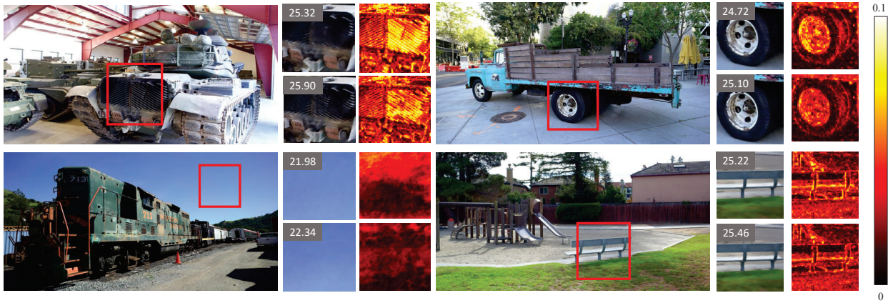
Figure 1: Error map of rendered images by NeRF++ [4] and our model in tanks and temples [1] dataset. The above and the below maps are generated error maps by NeRF++ and our model, respectively. For each subfigure, PSNR is shown on the upper left.
