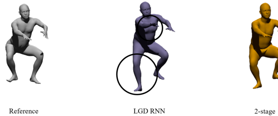
Figure 12: Denoising comparison. For this frame, the right lower leg sensor is missing in the input. LGD RNN struggles to reconstruct the pose (middle) whereas the two-stage approach does a better job (right). Notice how the missing sensor is affecting the entire pose output for LGD RNN.
