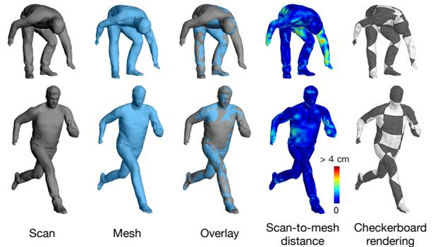
Figure 8: Our system can also infer clothed human body surfaces in consistent topology.
