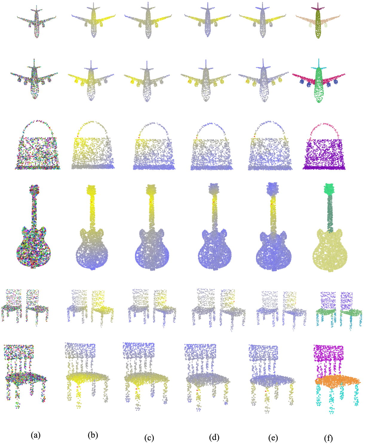
Figure 3: Visualization of the point distance across the accelerated network for part segmentation task. The distance of points to the red point in the figures is computed. Lighter color means closer distance. (a) The input shape. (b) Distance between points in the raw data. (c)-(e) Distance between point in the feature space from Layer 1, Layer 2, Layer 3 of the accelerated network. (f) Segmentation result. The accelerated network could still capture long-range dependency between points.
