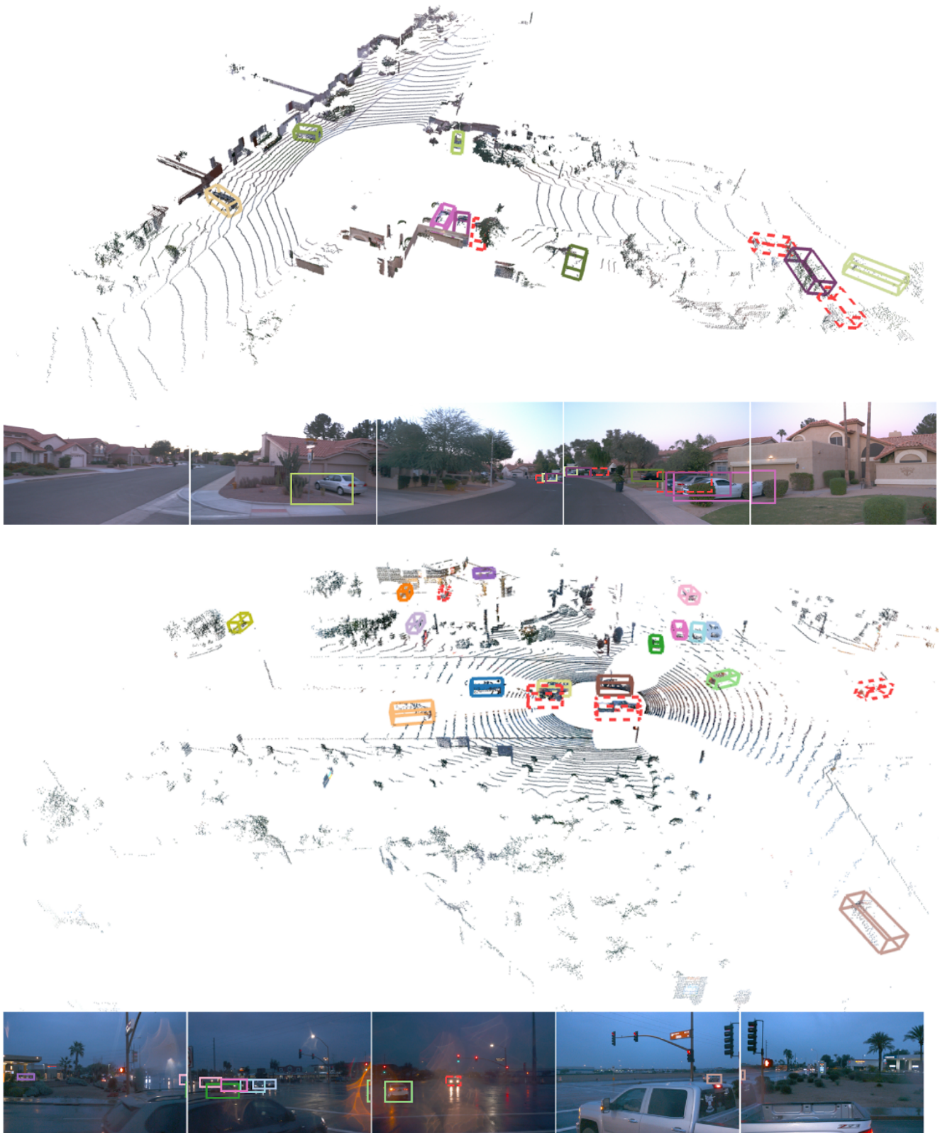
Figure 2. Failure cases examples: In these two challenging cases, the central image (stream) is not sufficient and a vehicle is missed.
