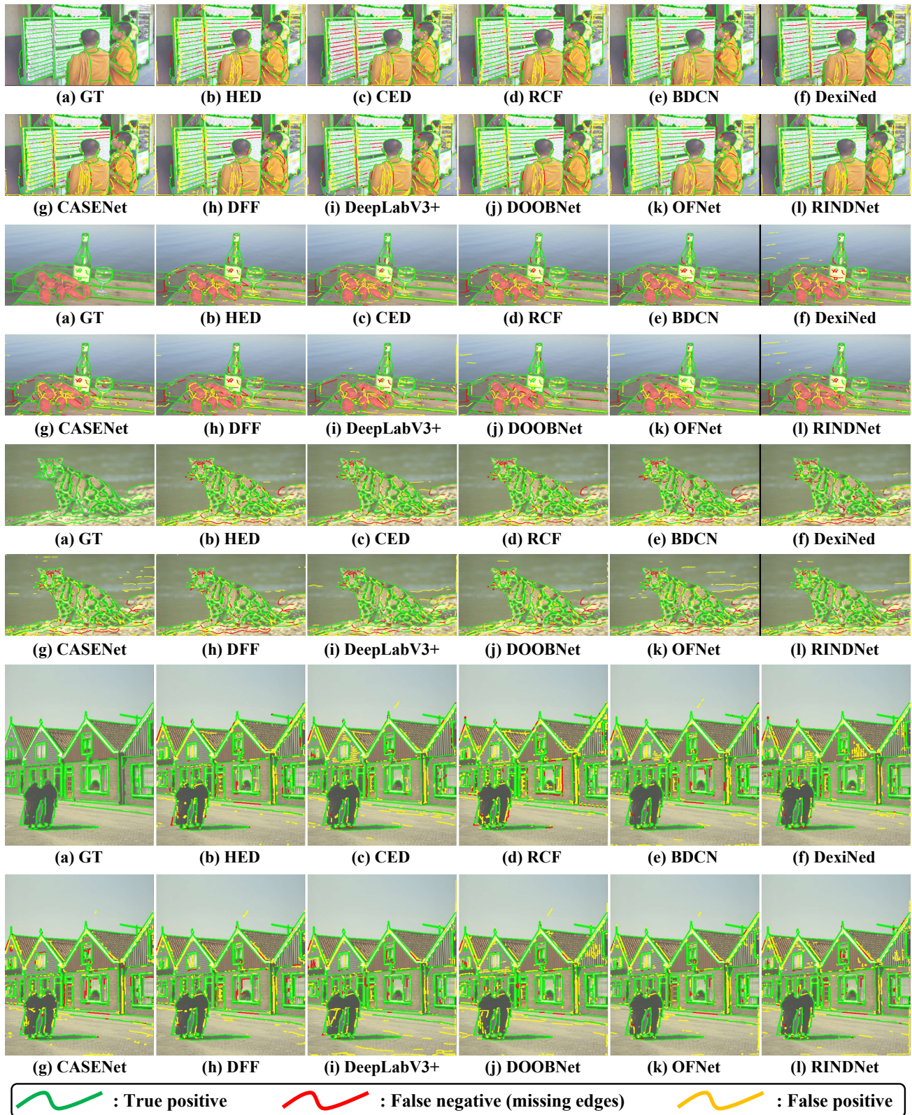
Figure 8. Qualitative comparison for Generic Edges (best viewed in color: “green” for true positive, “red” for false negative (missing edges), and “yellow” for false positive).
