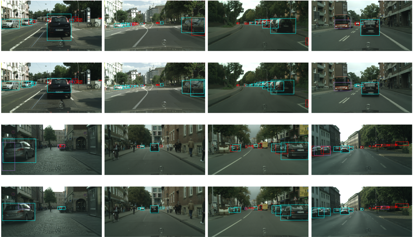
Figure 3. Qualitative results. Cross Camera scenario. Odd rows: Faster R-CNN and even rows: ViSGA (cosine). True positives, False positives and missed objects are shown as cyan, purple, and red boxes respectively.
