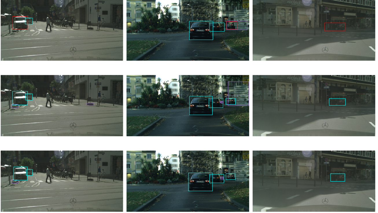
Figure 1. Qualitative results. Sim2Real scenario. First row: Faster R-CNN, second row: ViSGA (IoU) and, last row: ViSGA (cosine). True positives, False positives and missed objects are shown as cyan, purple, and red boxes respectively.
