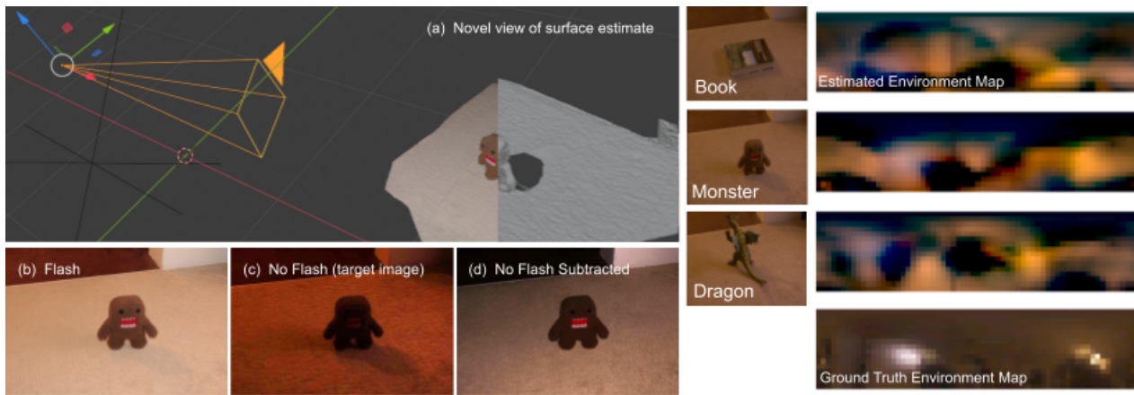
Figure 10. Estimation results from meshes obtained using photogrammetry. The left set of panels shows the capture and pre-processing approach: (a) Using photogrammetry, we obtain a camera pose, surface mesh, and diffuse texture. We capture two images (b) a flash image and (c) an image without a flash. (d) We use the flash-only image as input to the texture estimation using photogrammetry. On the right section, we use the approach on the left to recover the 3D geometry and diffuse texture of three objects: a book, monster, and dragon. For each of these objects we generate the corresponding ray transfer matrix and produce an estimated environment map. While the brightest sources can be identified in the estimated environment maps, the estimates appear to suffer from model mismatch, such as the warped recovery due to the larger dragon object and nearby light fixture. Addressing these failure modes is an area for future work.
