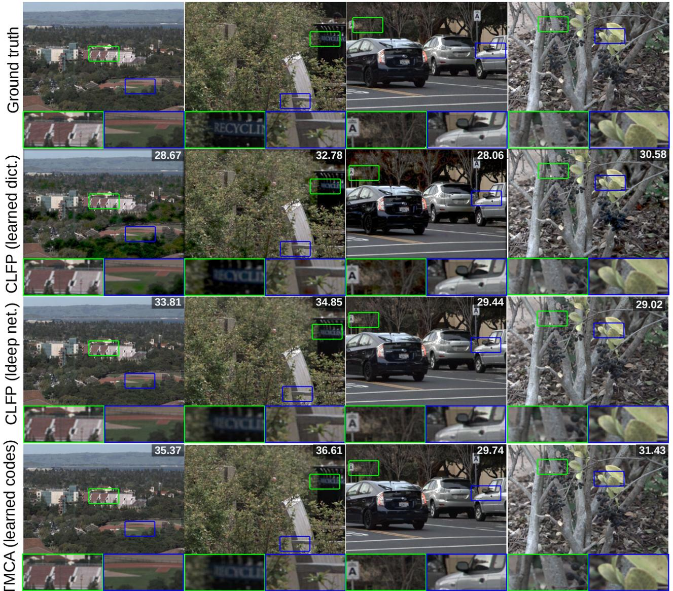
Figure 9. Additional light field results comparing our codification with TMCA using the deep network [2] as a decoder against (fourth row) the CLFP baselines with a sparse dictionary coding method as a decoder (second row) and the same codification also using the deep network architecture from [2] (third row). Numbers in the top right corner indicate PSNR compared to the ground truth (first row).
