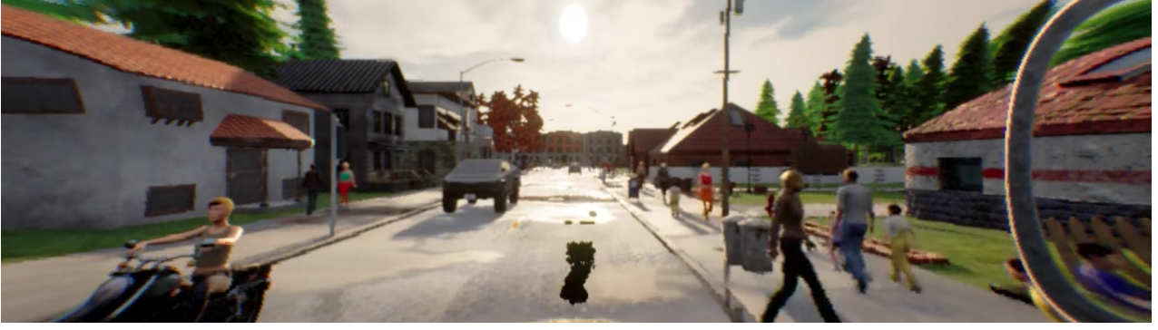
(a) Reflections from after-rain puddles in front of the ego-vehicle are incorrectly rendered as black pixels.
