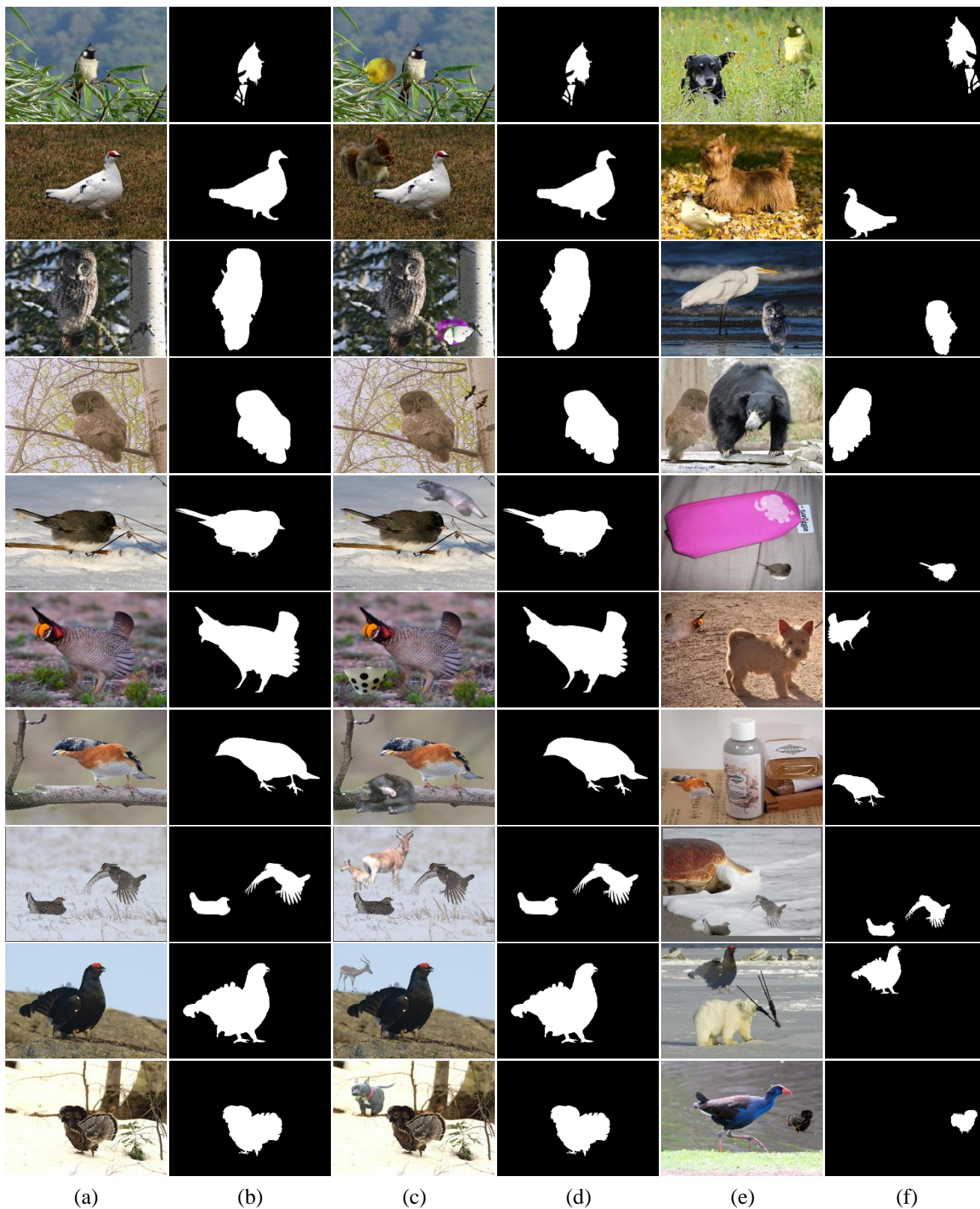
Figure 3. More synthesized examples of our proposed data synthesis strategies. (a) original images. (b) original ground truth. (c) normally synthesized images. (d) ground truth for the normally synthesized images. (e) reversely synthesized images. (f) ground truth for the reversely synthesized images.
